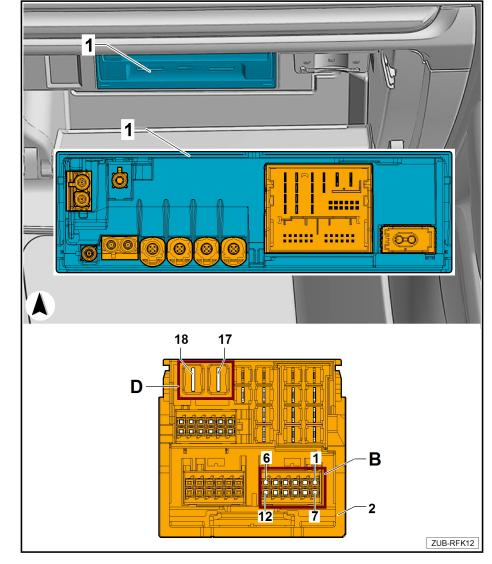
versing camera wiring harness into the free compartment -18- in connector -2 area D-.
